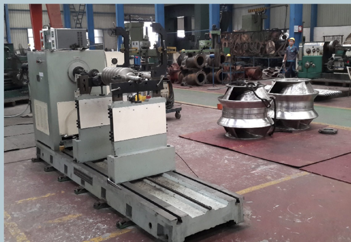
采用上海申克制造的动平衡设备，保证了产品的平衡运行。 Adopt dynamic balance facilities from Shanghai Shenke Manufacturer to make sure the operation of the dynamic balance test.
